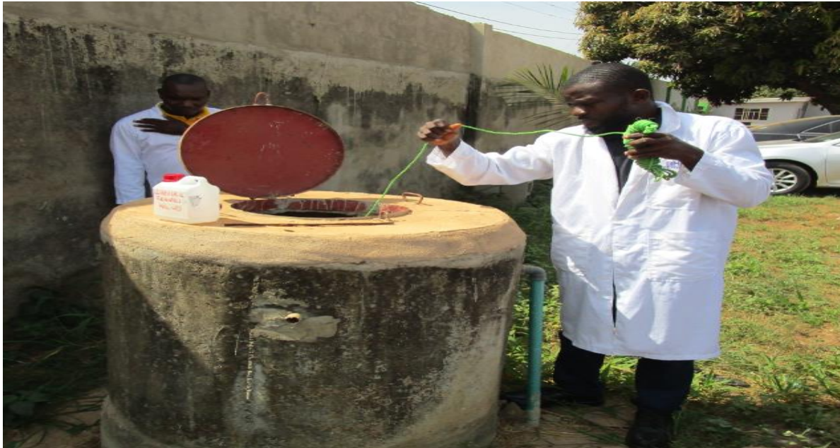
PLATE4.3 : CONSULTANTS CONDUCTING GROUND WATER SAMPLING
