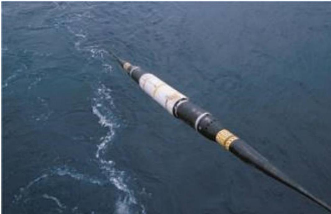
**Plate 3.3: A Typical Repeater (Source: ASN, 2020)**
