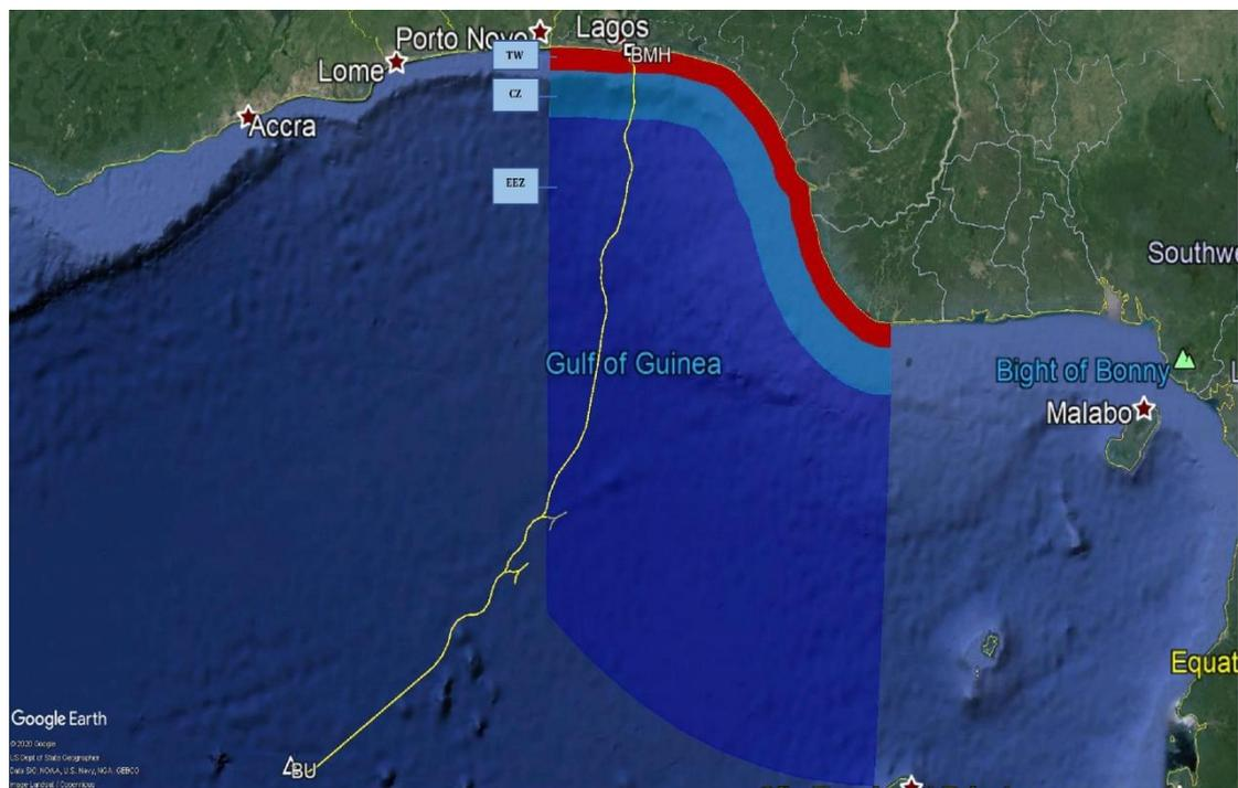
**Figure 1.4: Nigerian maritime boundaries showing the EQUANO Nigeria submarine cable route (Source: Adapted from Google Map, 2020)**
