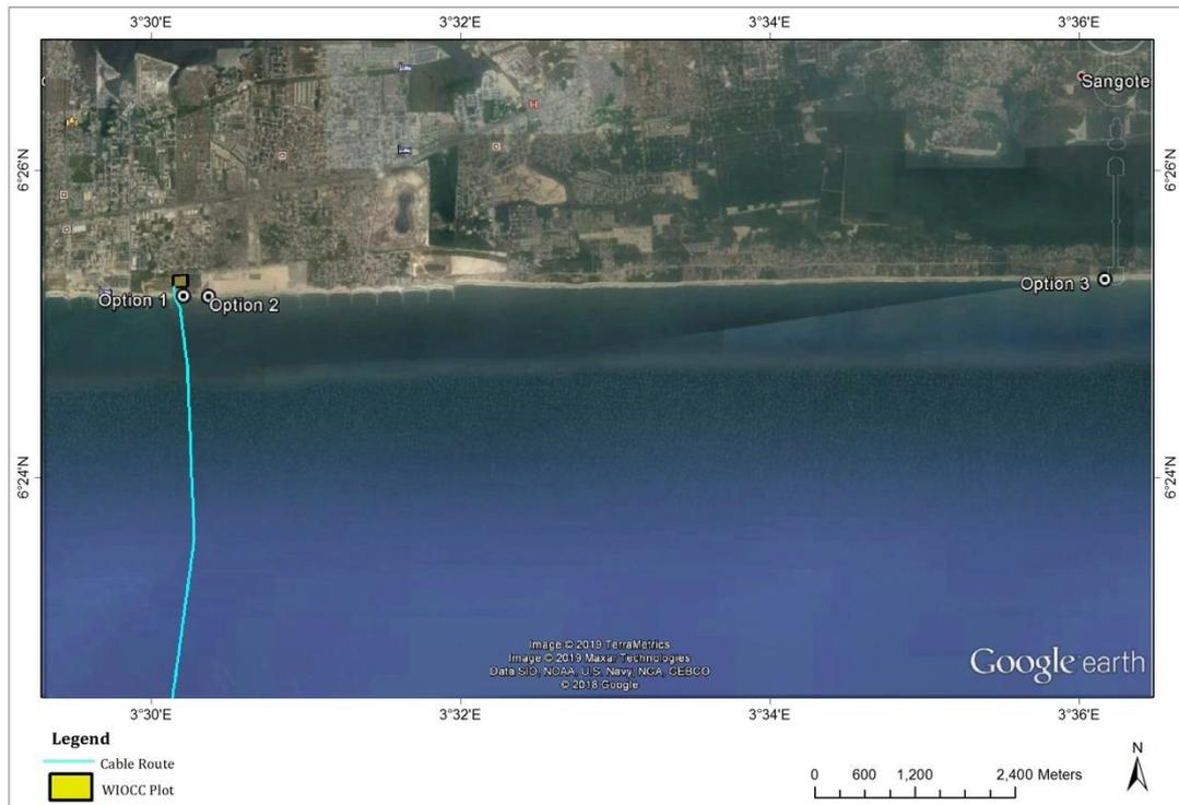
**Figure 2.1: Site options considered for cable landing point and associated coastal infrastructure, showing the offshore cable seaward of the connection to the BMH at Option 1 (Source: Adapted from Google Map, 2019)**
