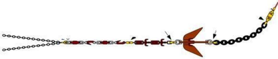
**Figure 3.8: Typical grapnel tool for removing seabed debris prior to plough burial operation**
