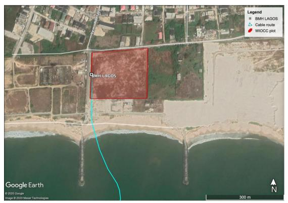
Figure 3.4: Proposed EQUIANO Nigeria submarine cable route up to the BMH location within the WIOCC plot (red box) at Elegushi beach, Lagos (Source: Adapted from Google Map, 2020)
