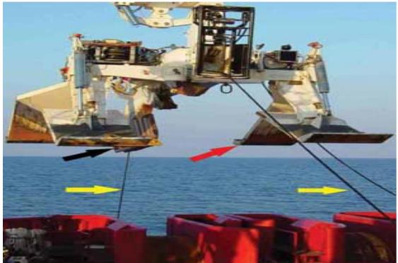
Plate 3.4: A typical sea plough about to be deployed from a cable ship. The fibre-optic cable (yellow arrows) is fed into a furrow cut by the plough-share (black arrow), which is towed across the seabed on skids (red arrow) (Source: Carter et.al; 2009)
