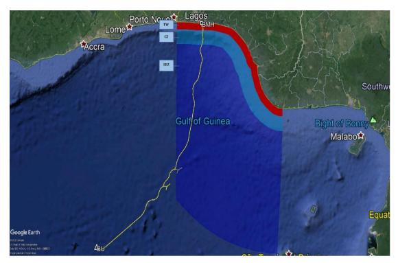
Figure 1.2: Proposed EQUIANO Nigeria submarine cable route from BU (BU NGA) to the proposed BMH in Lagos (Source: Adapted from Google Map, 2020)
