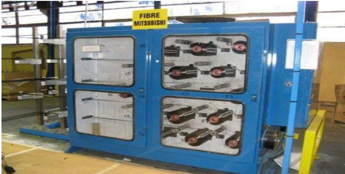
FIG 3.2: A TYPICAL CREEL USED IN FILAMENT WINDING
