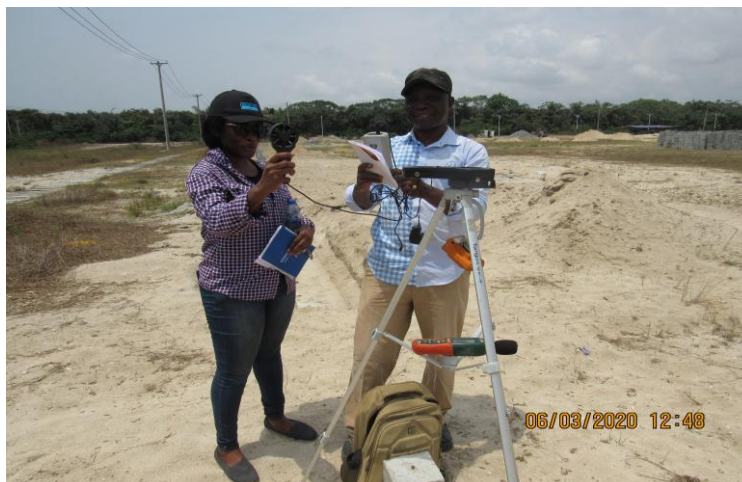
Plate 4.8: Typical Air Quality/Noise Monitoring Setup during the Study (Photographed March 2020)
