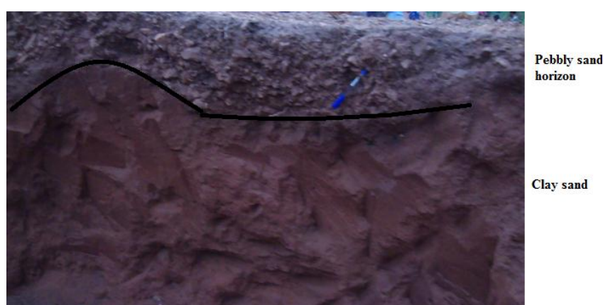
Plate 3.6: Soil profile obtained from a cut section in Ehanlen community, Ewu (6.80148°N, 6.24710°E; Scale: Pen 15.5 cm long)
