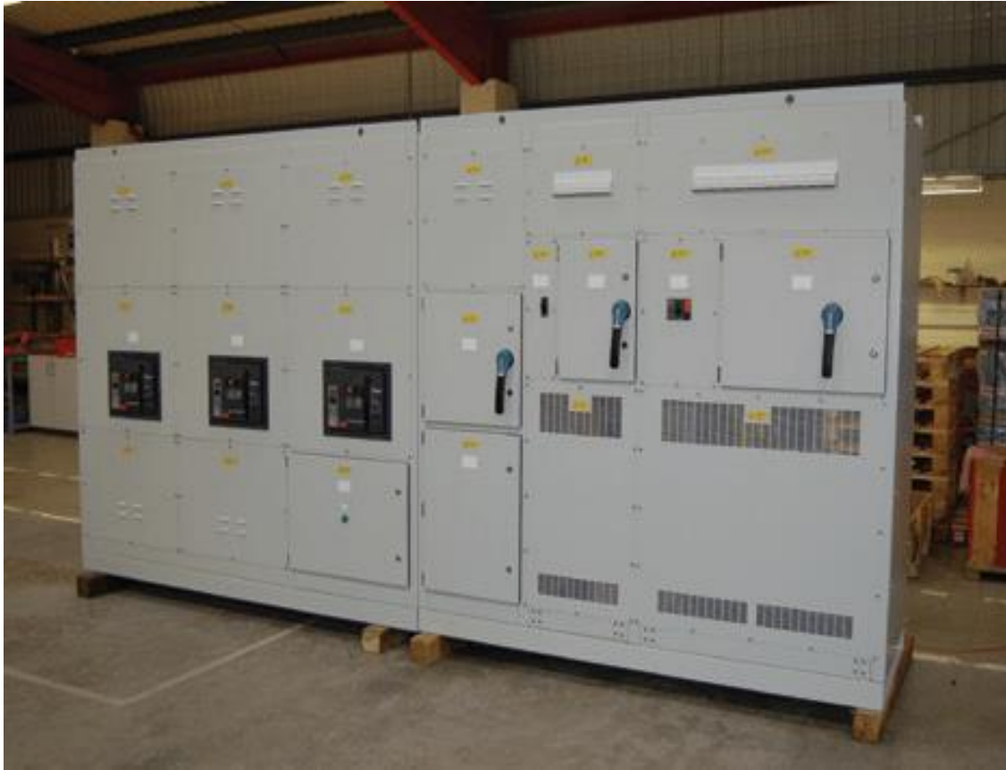
Plate 3.2: A typical low voltage switchgear cabinet
