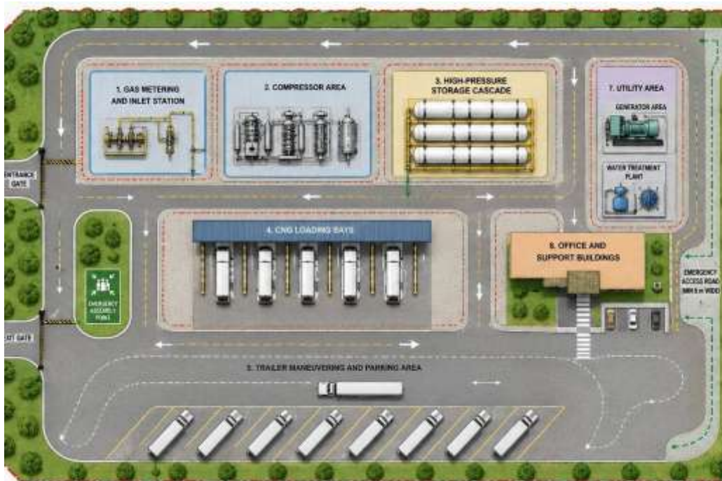
Plate ES-1: Aerial view of a comparable CNG Mother Station — multi-stage compressor skids, high-pressure cascade storage banks, and loading manifolds
