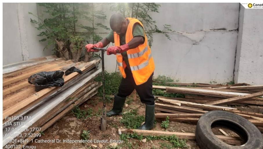
Plate 4.4: Soil sampling at the proposed Radio FM station Site (Source: FIX FM Field Studies, April 2026)
