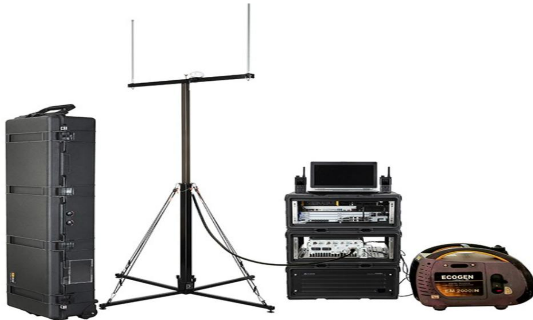
Figure 3.6: Trunked Radio System I
