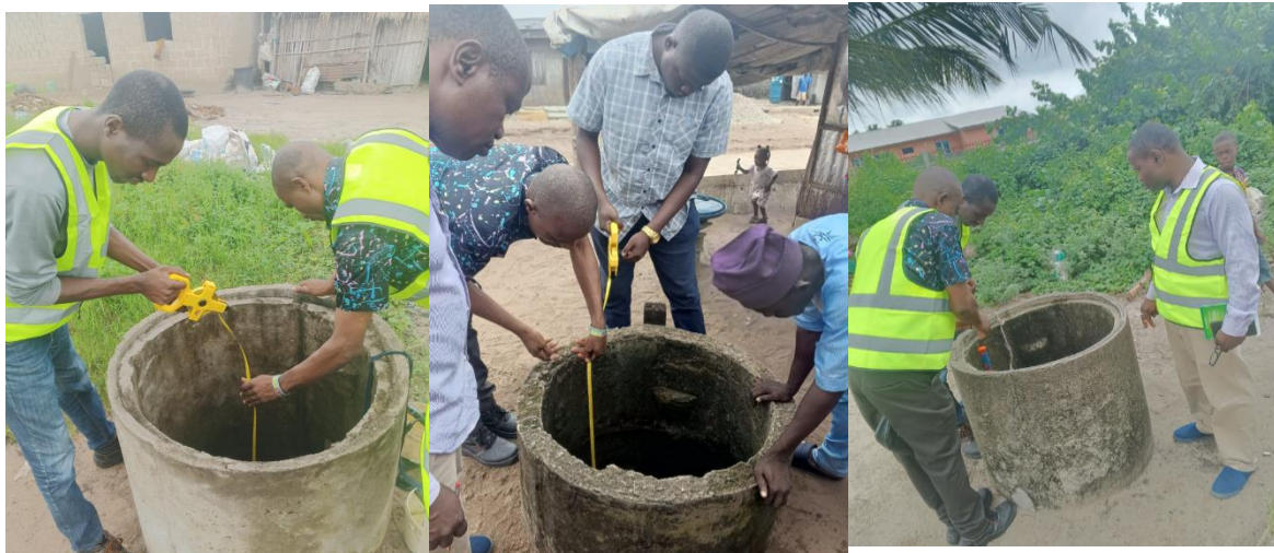
Fig. 4.22: Water level measurement at different locations in the study area Geophysical Survey (VRT and ERT)
