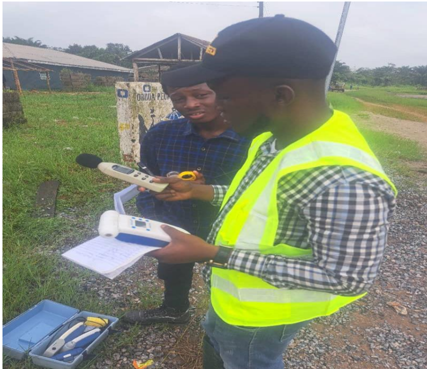
Plate 4.3: Noise Level Measurement with the aid of Extech Noise Meter
