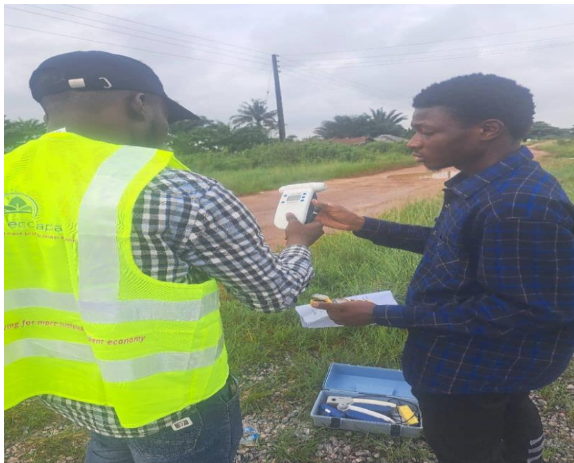
Plate 4.2: Air Quality Measurement with the aid of Aeroqual Series 500
