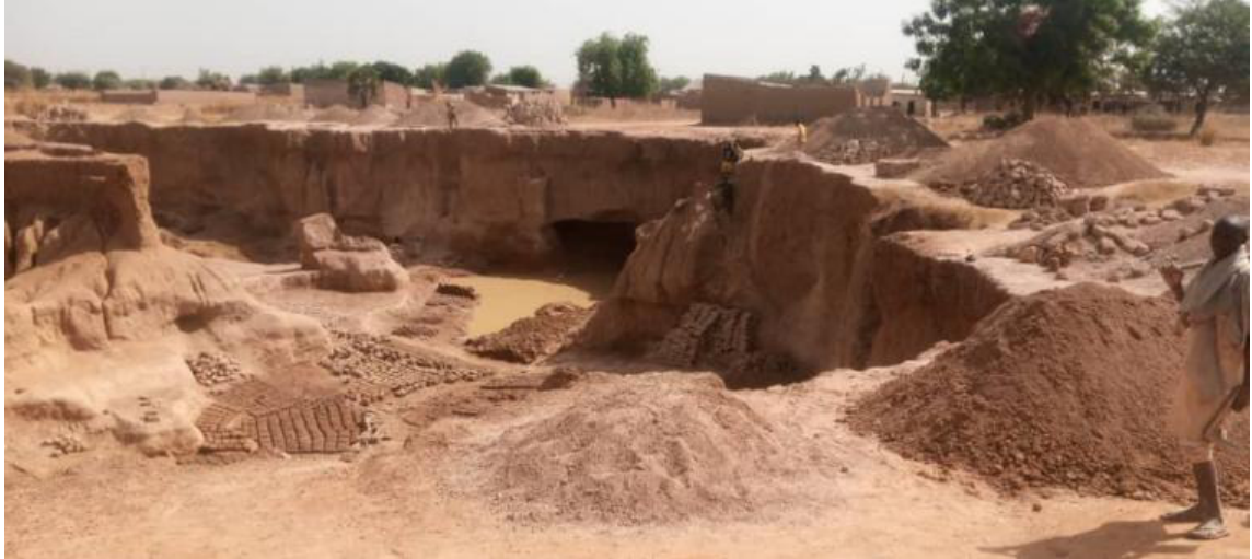
Plate 4. 45: Mud Sand Excavation area for mud building blocks, at Kwidawa, LGA: Dawakin Tofa, Kano State
