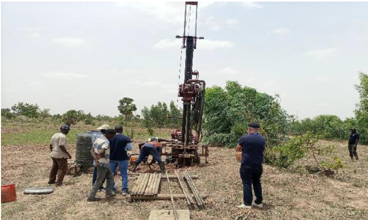
Plate 4. 21: Rotary drilling and rock coring process during geotechnical survey (Source: Liscon Geotechnical Limited, 2021)
