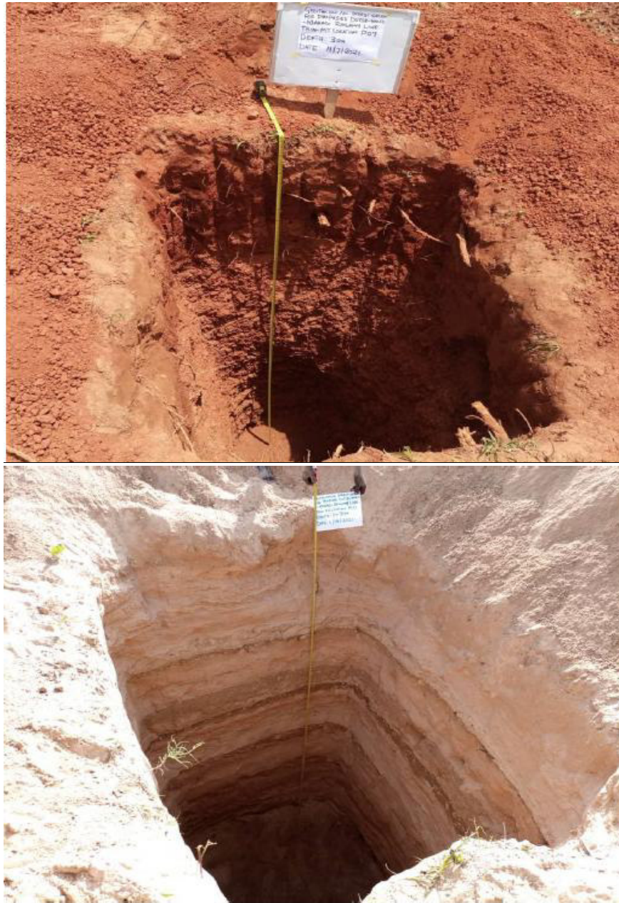
Plate 4. 22: Some of the trial pits excavated during geotechnical study
