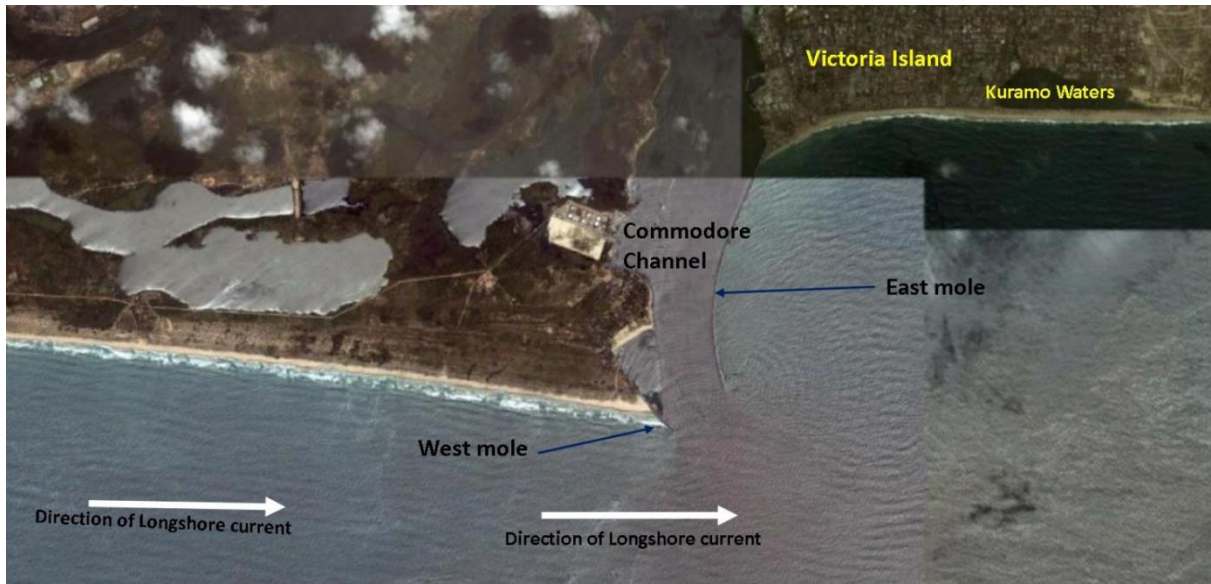
Plate 4.3: East and West Moles with the Prevailing Long shore Current Direction Source: Nwilo, Ibe, Adegoke and Nwabufo (2020) -Google Earth, October 2002
