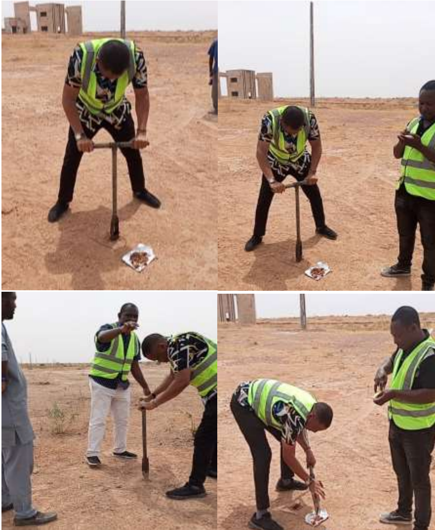
Plate 4.4: Soil sample collection using soil auger
