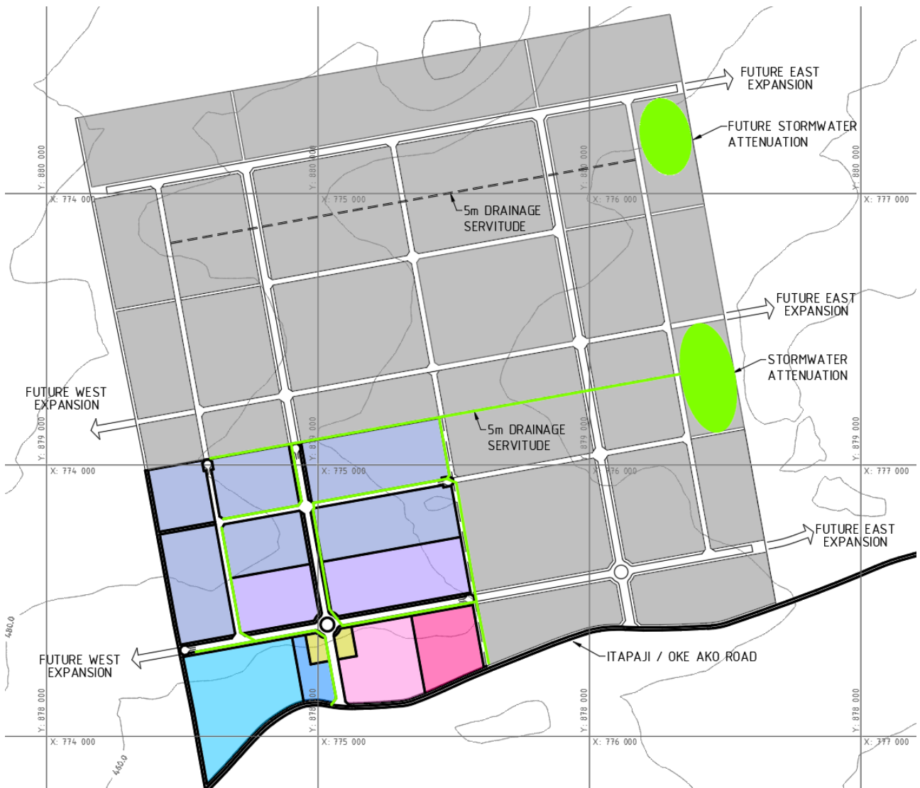
Figure 3.26: Stormwater Management Plan Source: (Surbana Jurong & SMEC, 2022)
