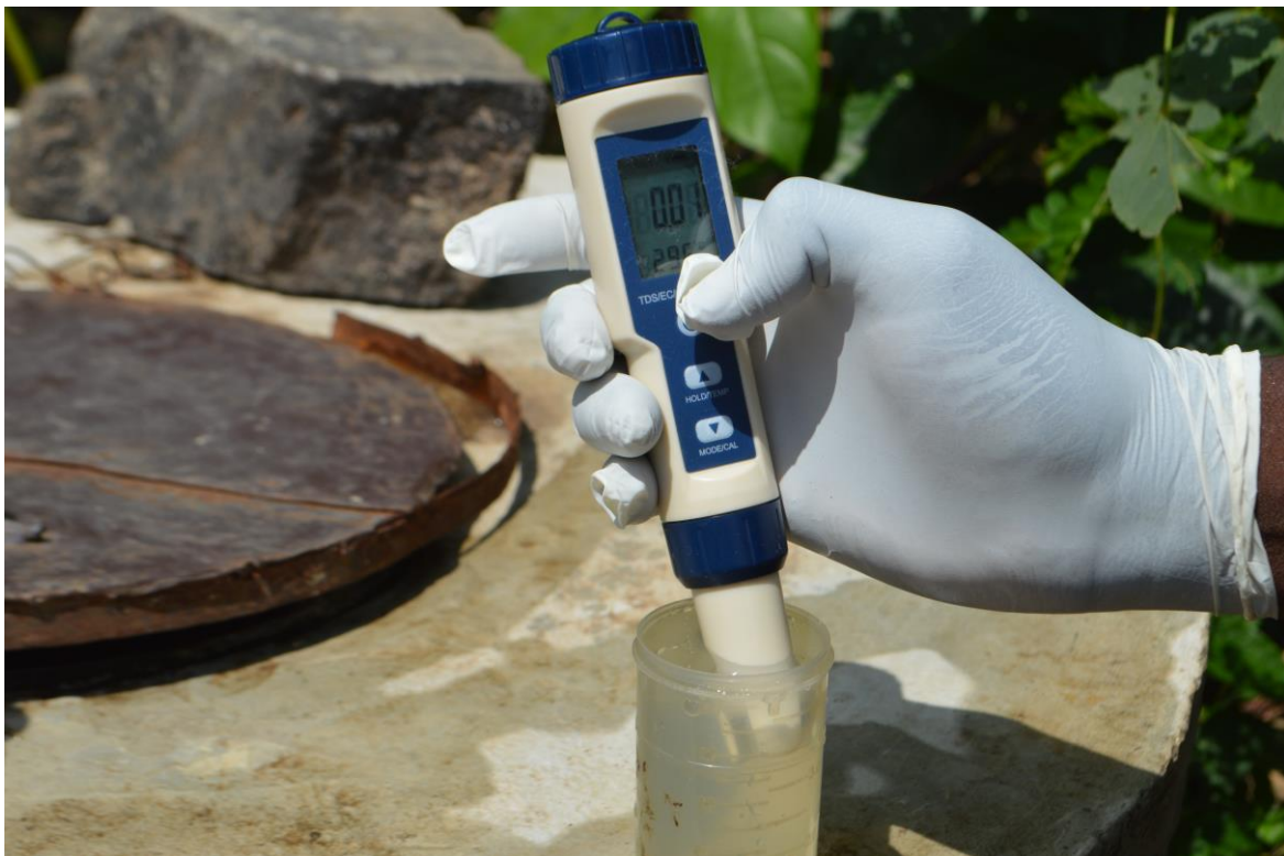
Photo 4.15: In-Situ Testing of Ground Water Sample Source: (Field Survey, November 2021)
