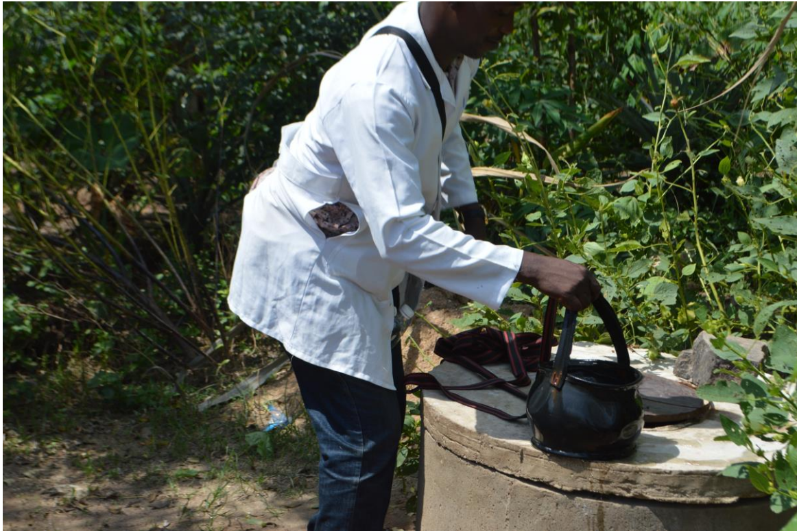
Photo 4.14: Collection of Ground Water Sample Source: (Field Survey, November 2021)
