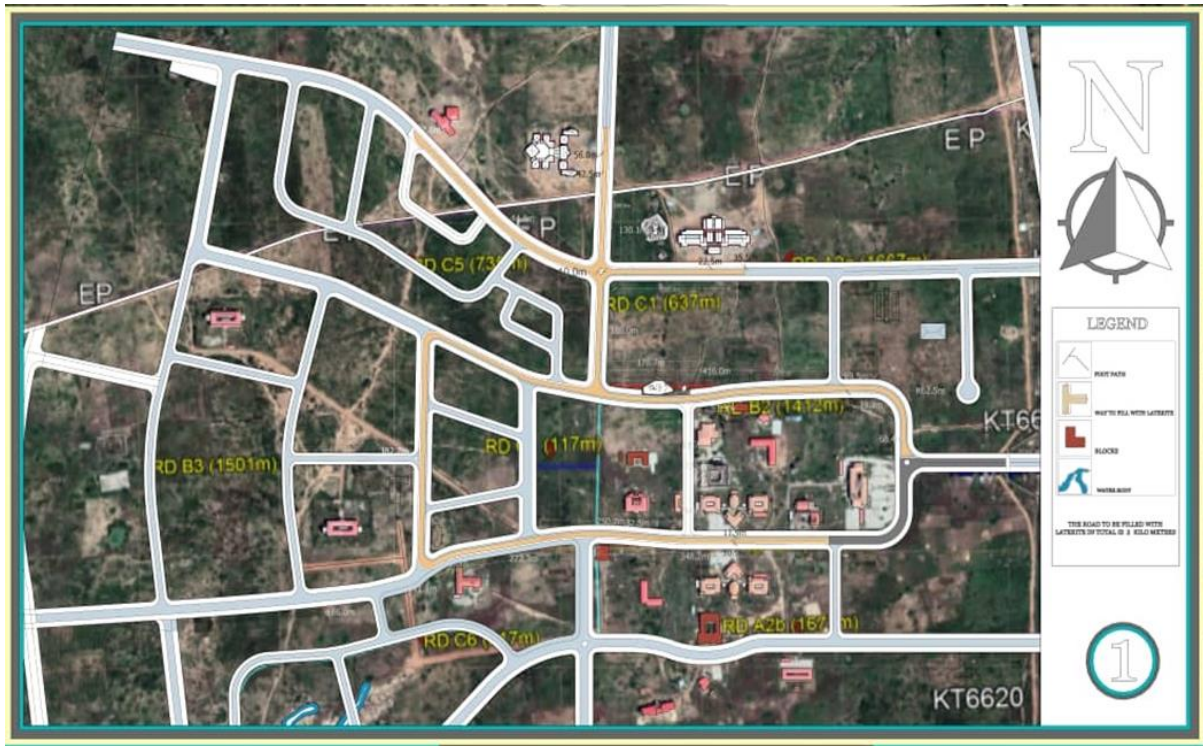
Figure 3. 15: Planned Road Network in FUDMA (Source: REA EEP 3 Front-end and Engineering Design)
