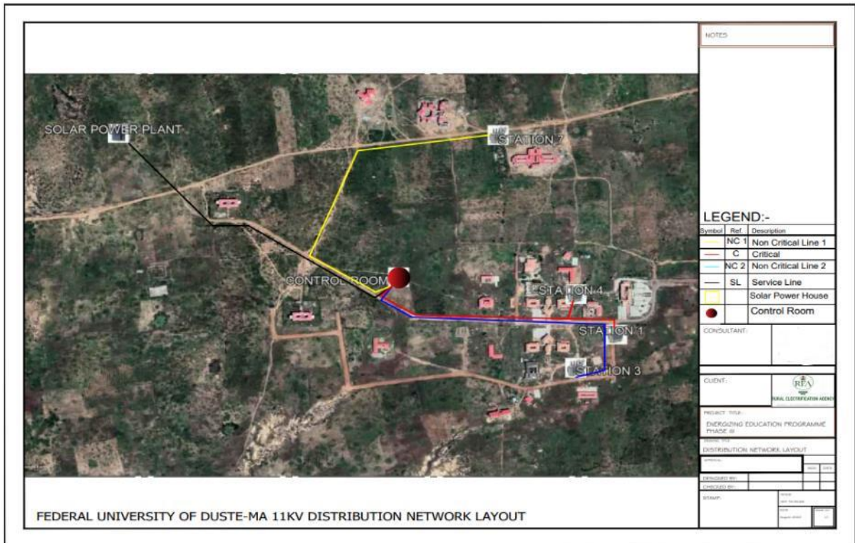
Figure 3. 12: Distribution Network Layout for FUDMA (Source: REA EEP 3 Front-end and Engineering Design)
