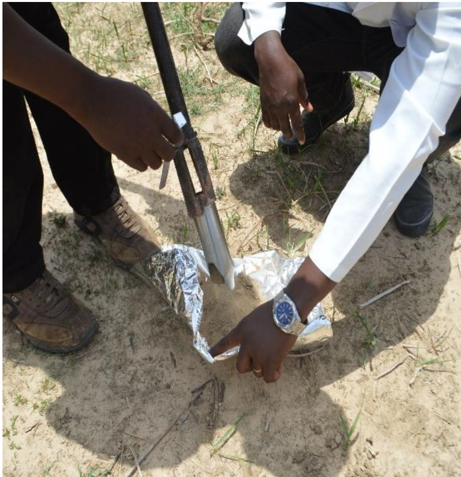
Plate 4.19: Bagging of soil samples by lab scientist and his assistant Source: Envicons Field Survey, 8th July, 2021
