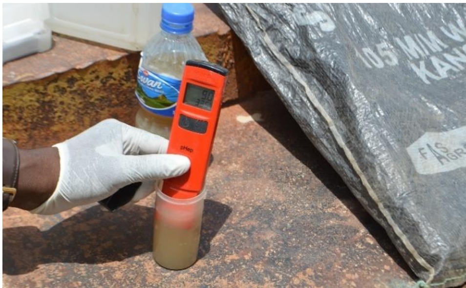
Plate 4.16: In-situ Measurement of Borehole Water Sample Parameters
