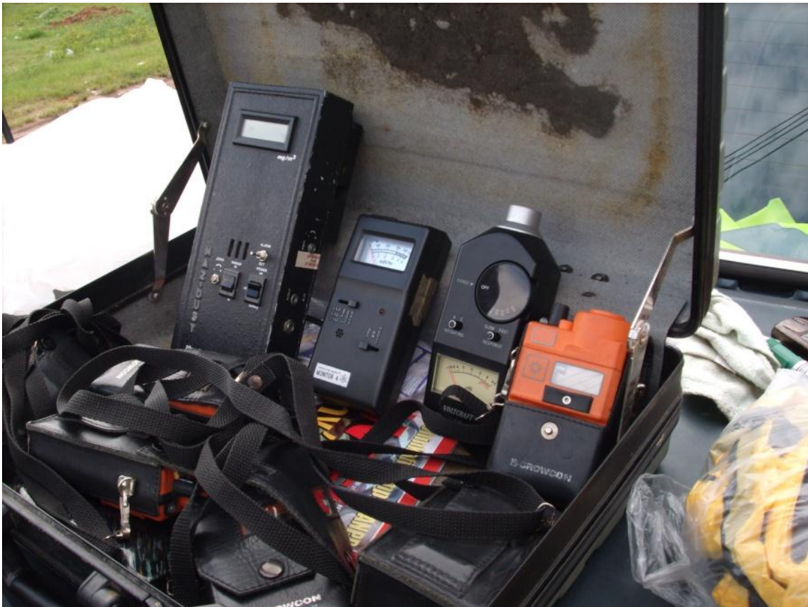
Plate 4.1: Showing air quality monitoring equipment during the studies
