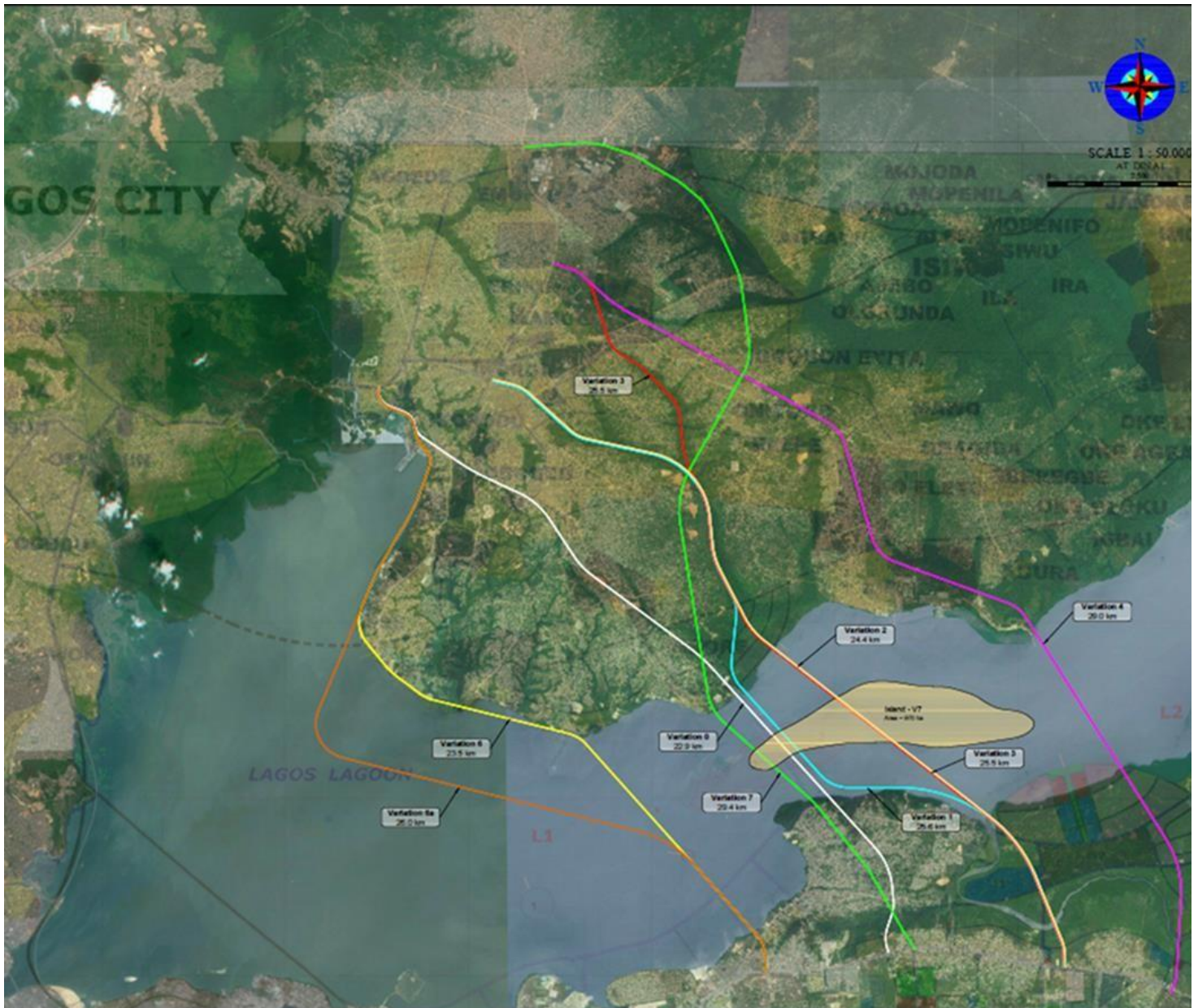
Figure ES 1: Some of the Alternative Alignments considered for the 4 th Mainland Bridge Project
