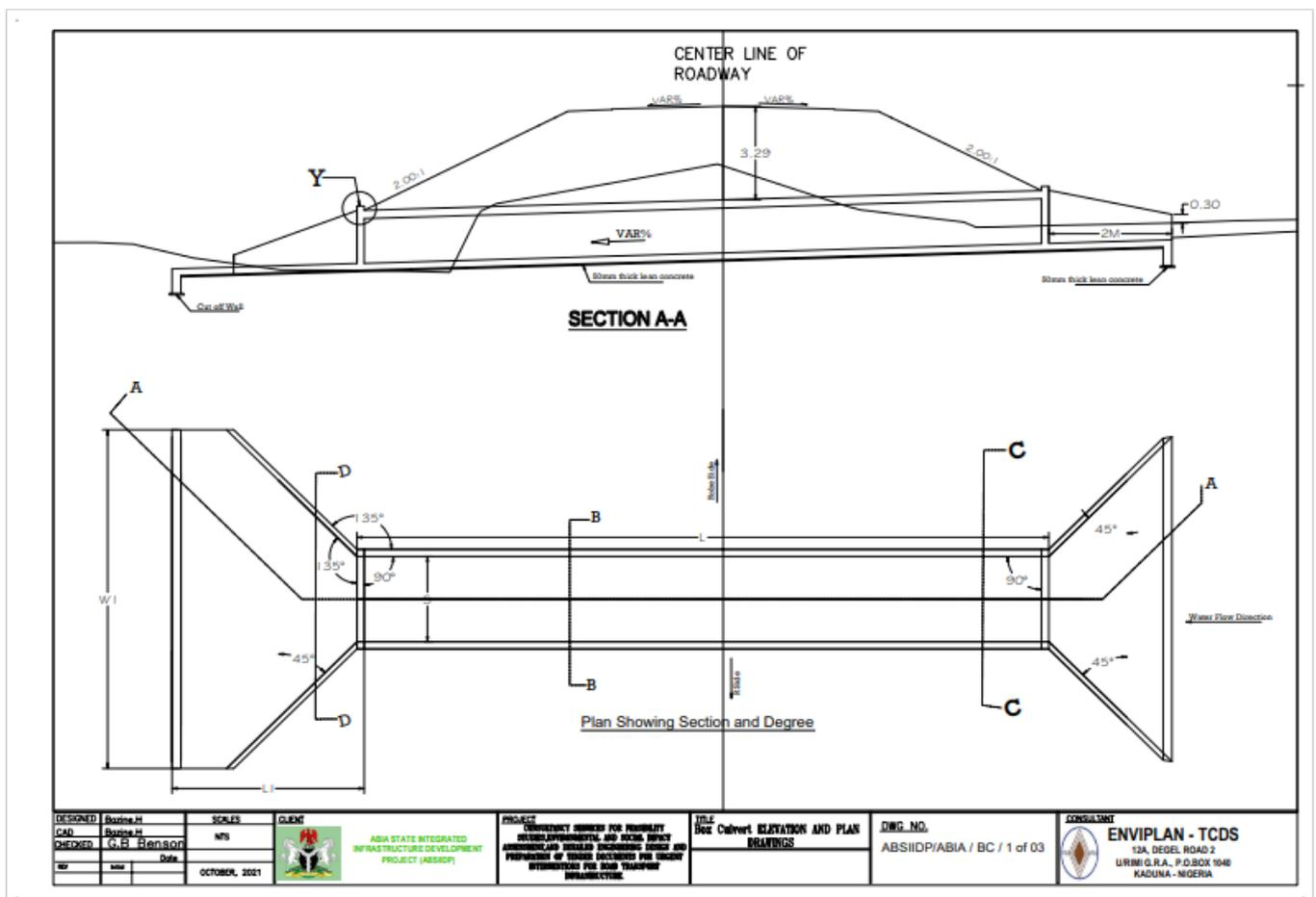
**Figure 3.2 Box Culvert In Let And Out Let 01**
