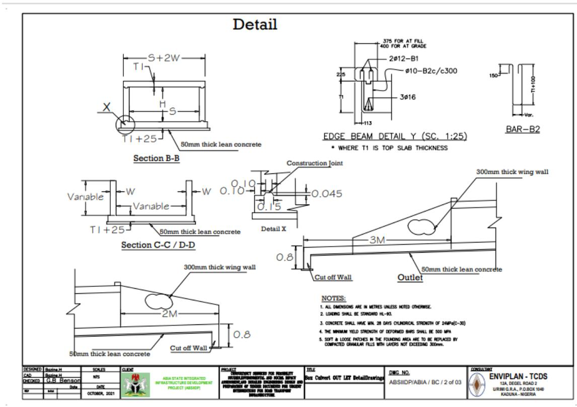
Figure 3.1 Box Culvert In Let And Out Let 02
