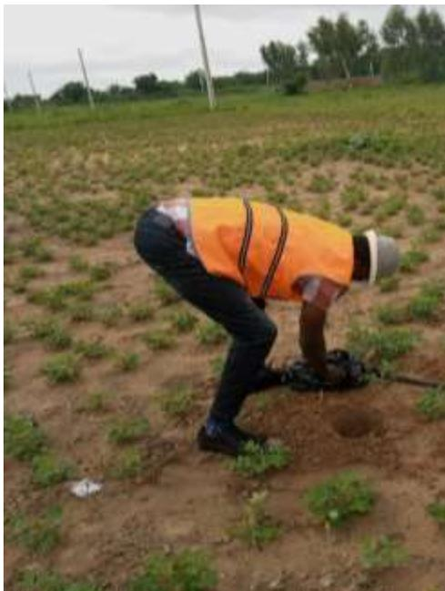
*Fig 8: Soil sample collection from the proposed site*
