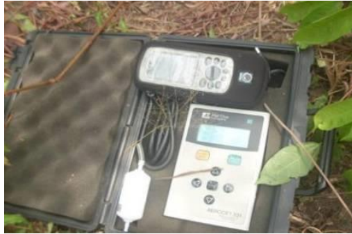
Plate 4.2: Pictures of some in-situ digital meters used to measure ambient air conditions
