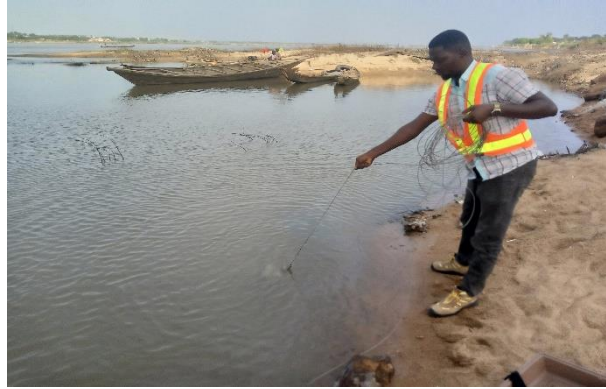
Plate 4.21: Sediment sampling with grab in River Benue
