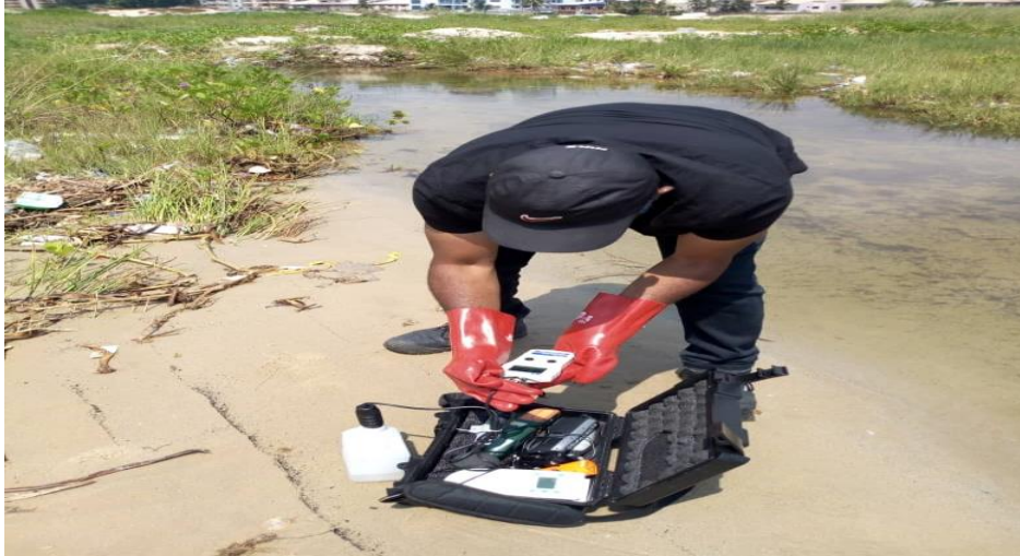
Plate 4.2: pH meter being used for in situ measurement of water quality
