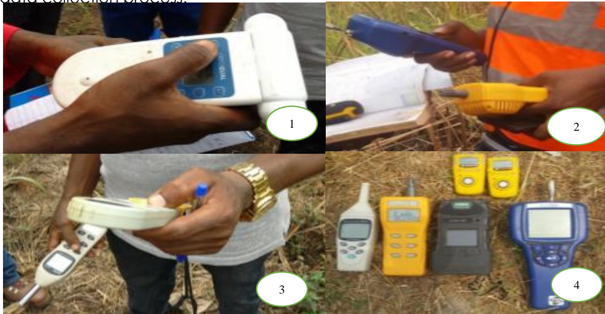
Plate 4.1a: In Situ Meters - 1: Aeroqual multi gas meter, 2: GPS, Aero Track Handheld Airborne Particle Counter (SPM), 3: Noise Meter and Weather tracker and 4: SO 2 meter, NO 2 meter, H 2 S meter etc.
