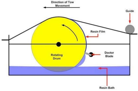
FIG 3.3: DIAGRAM SHOWING THE TOW IMPREGNATOR
