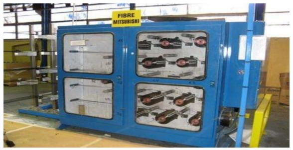
FIG 3.2: A TYPICAL CREEL USED IN FILAMENT WINDING
