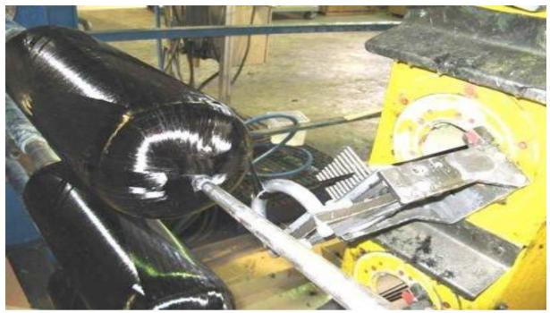
PLATE 3.0: WIND HEAD - WET PROCESS
