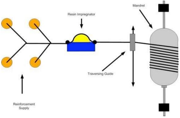
FIG. 3.1 : DIAGRAM OF FILAMENT WINDING SET UP FOR CYLINDER PRODUCTION
