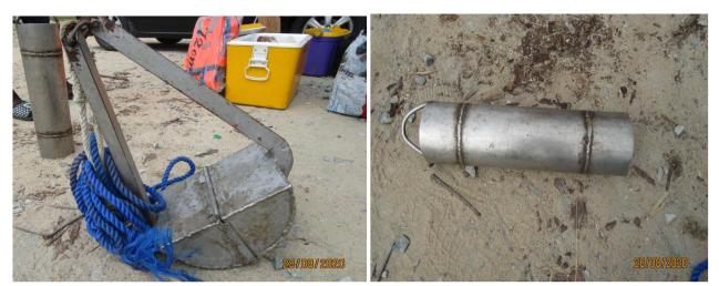
PLATE 4.27: SEDIMENT SAMPLER (GRAB)
