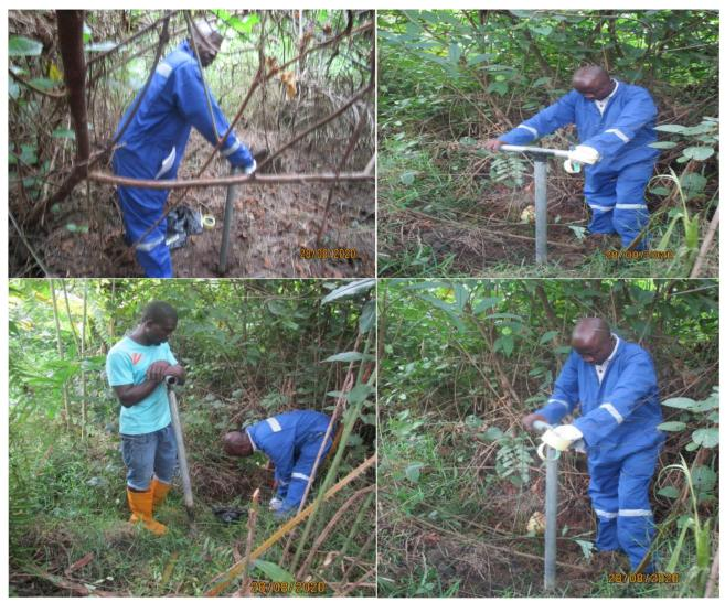
PLATE 4.3 : CONSULTANT REPRESENTATIVE CONDUCTING SOIL SAMPLING WITH HAND AUGER
