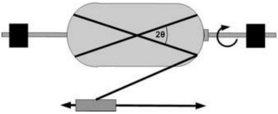
FIG 3.4: HOOP AND HELICAL WINDING CONFIGURATIONS
