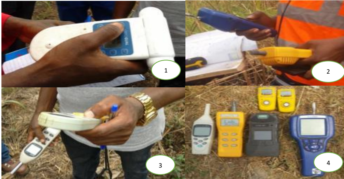
Plate 4.2a: In Situ Meters - 1: Aeroqual multi gas meter, 2: GPS, Aero Track Handheld Airborne Particle Counter (SPM), 3: Noise Meter and Weather tracker and 4: SO 2 meter, NO 2 meter, H 2 S meter etc.
