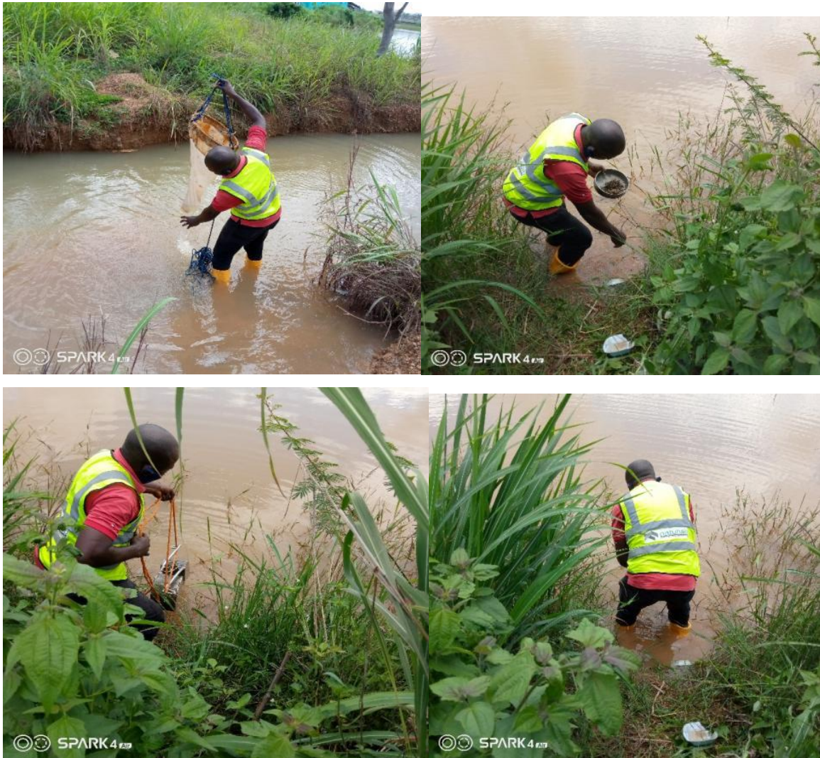
Plate 4.4: Sampling of Sediment Plankton, Zooplankton and Benthic Macroinvertebrates
