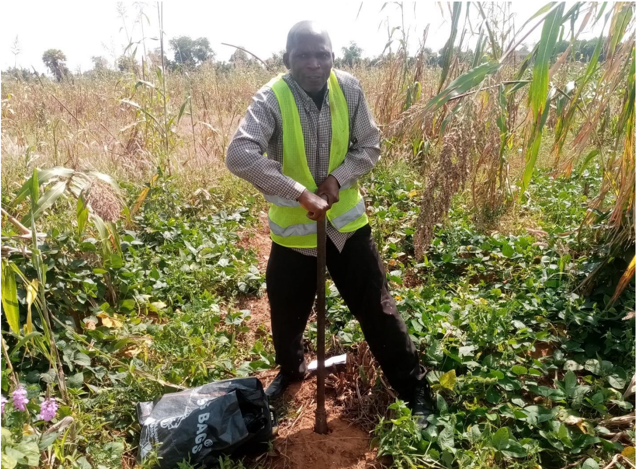
Plate 4. 1: Soil being sampled on the proposed factory site
