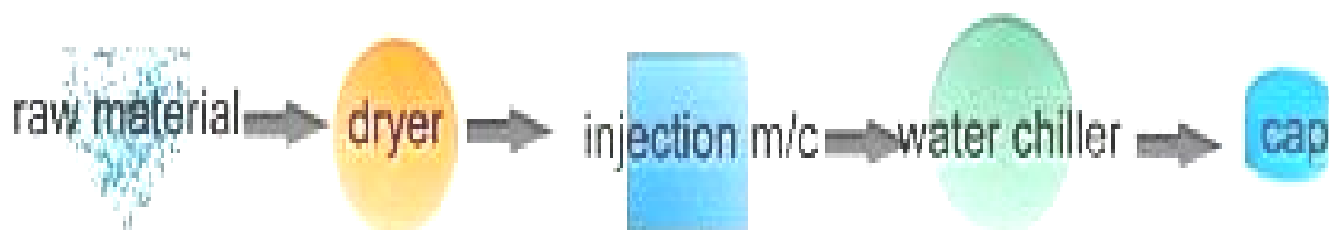
Fig 3.4 The flow chart of plastic injection molding
