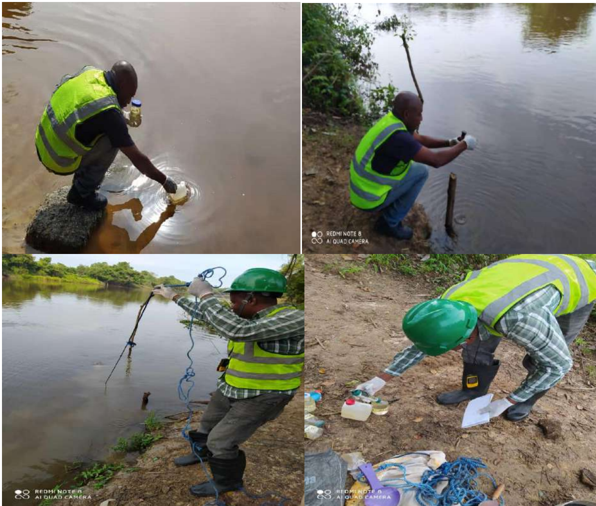
Plate 4.2b: Sampling of Surface water and using of pH meter for in situ measurement of the water quality
