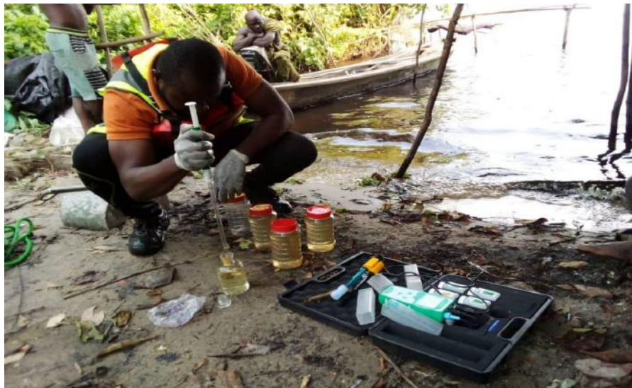
Plate 4.11: Preservation of Surface Water Sample with high grade analytical Preservatives
