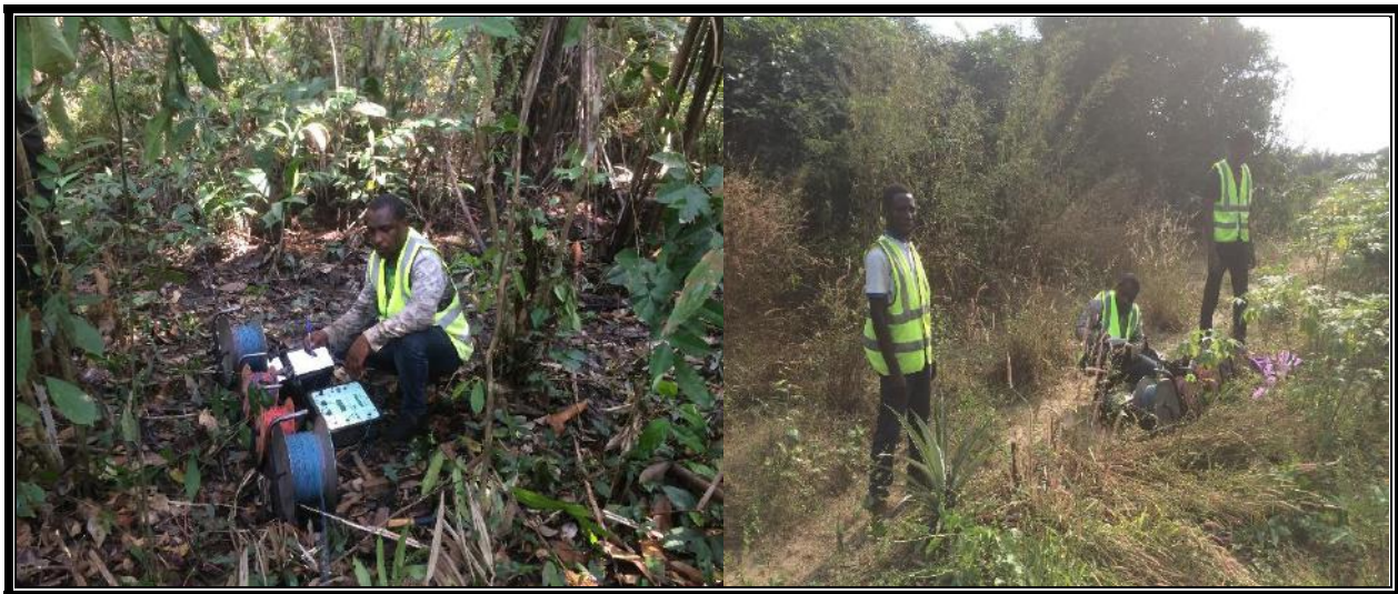
Plate 4.5: Geophysical Acquisition Team Collecting Data at VES Sampling Point using PASI Terrameter and its Accessories
