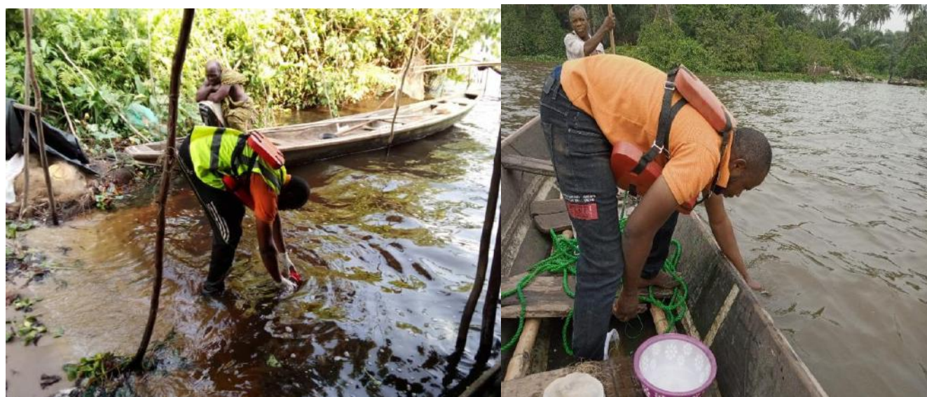
Plate 4.10: Sampling at the lagoon by direct water sample collection
