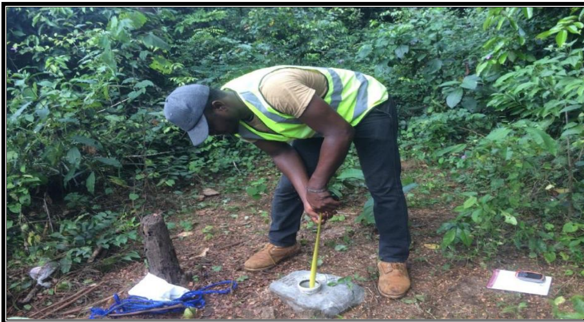
Plate 4.6: Picture of the Field Staff taking Static Water Level Measurement with Graduated Steel Meter Tape at Borehole 2 (BH2)
