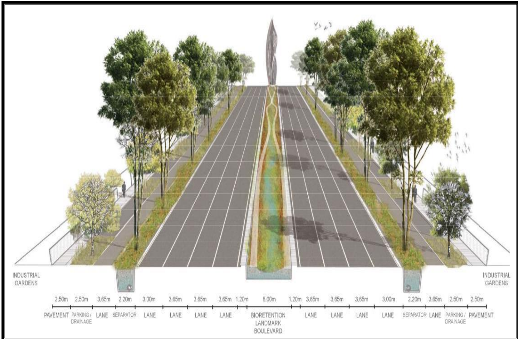
Figure 3.10: Section through the Primary Road
