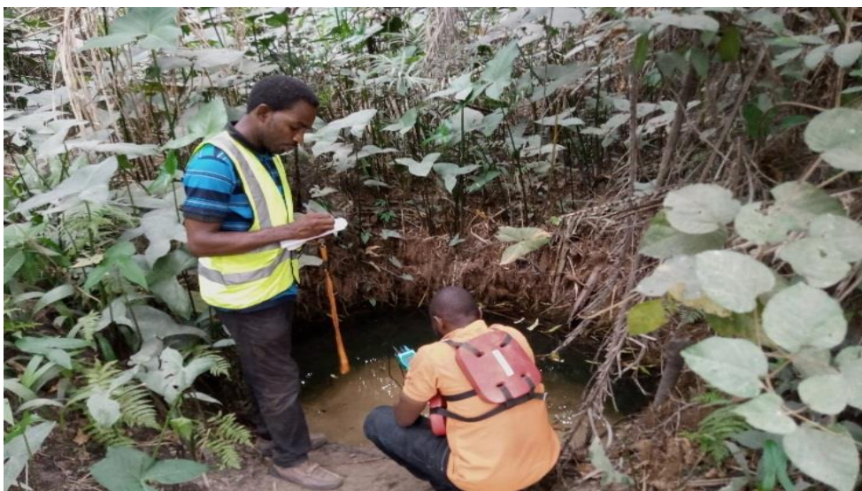
Plate 4.13: Ground water sample collection and in situ measurement.
