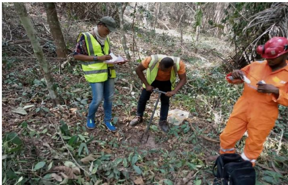
Plate 4.15: Soil sample collection using soil auger
