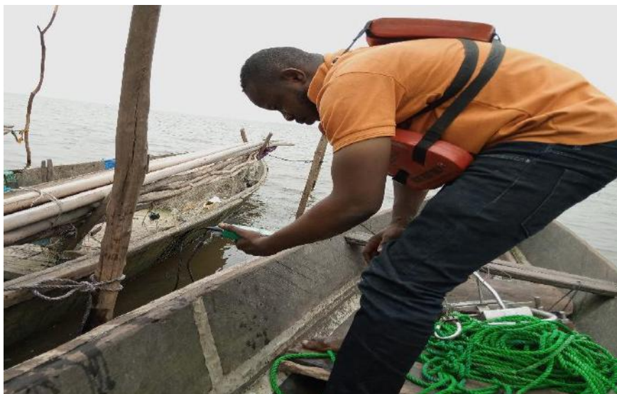
Plate 4.12: In situ measurement of unstable parameter using Apera water meter SX823-B Model
