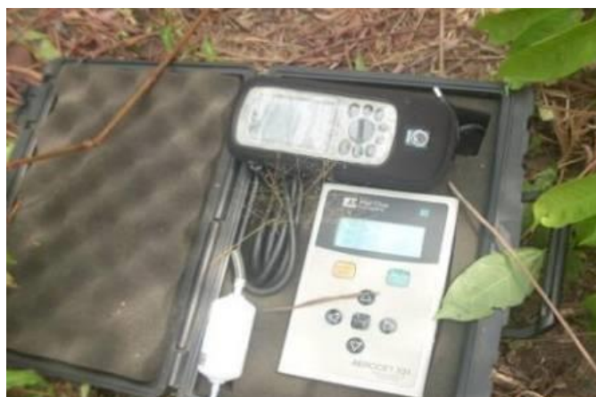
Plate 4.1: Pictures of some in-situ digital meters used to measure ambient air conditions
