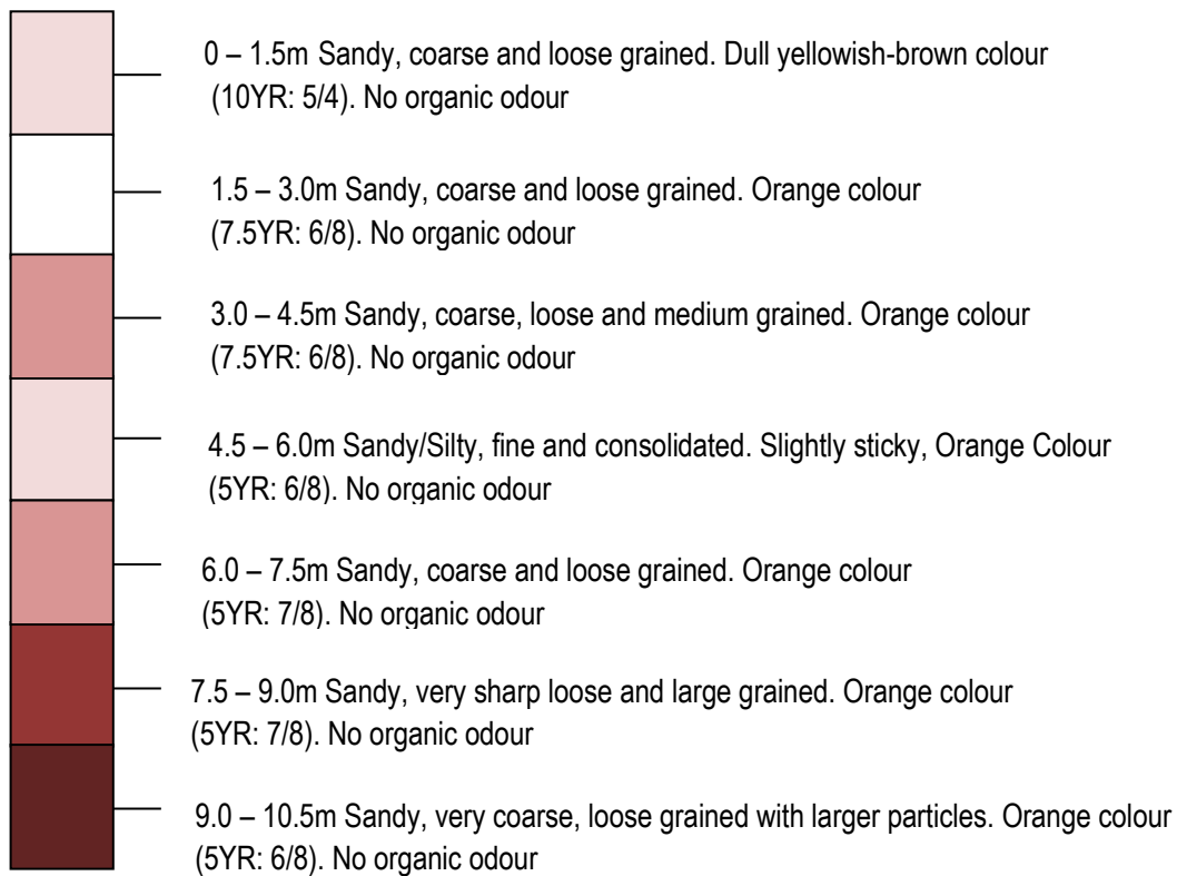
Figure 4.27: Schematic Section of Soil Profile at the Study Area
