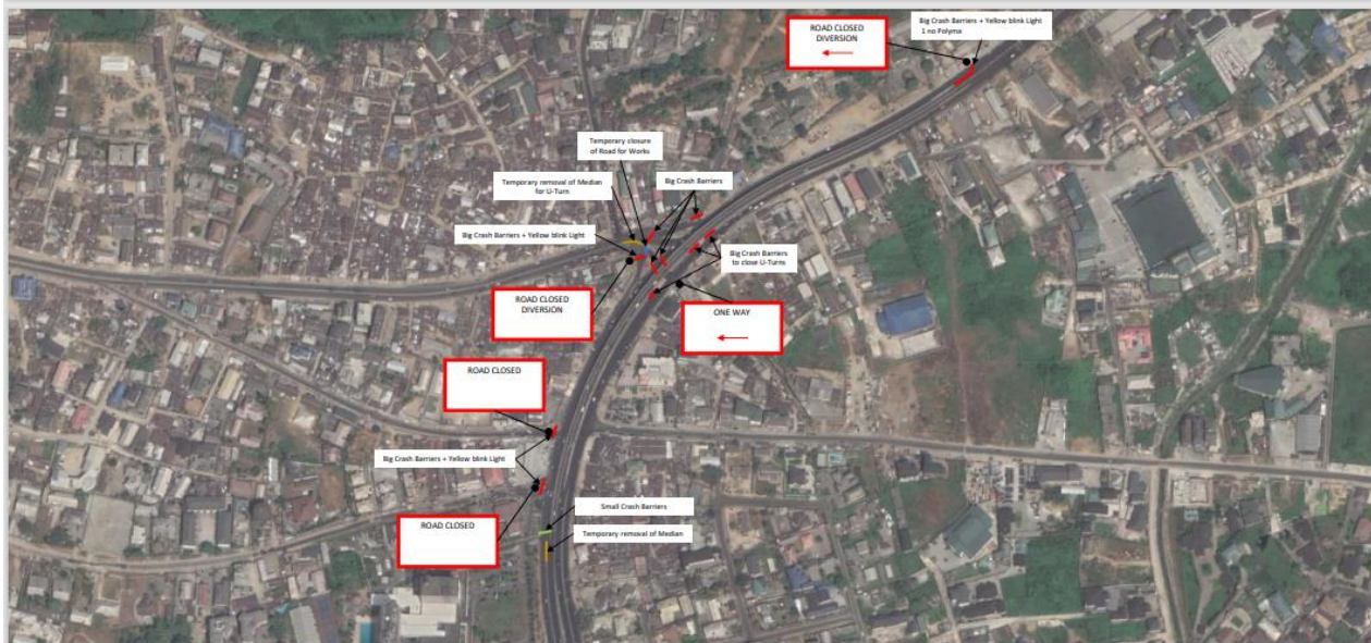
Figure 7.2: Traffic Diversion Plan for Rumuola Flyover
