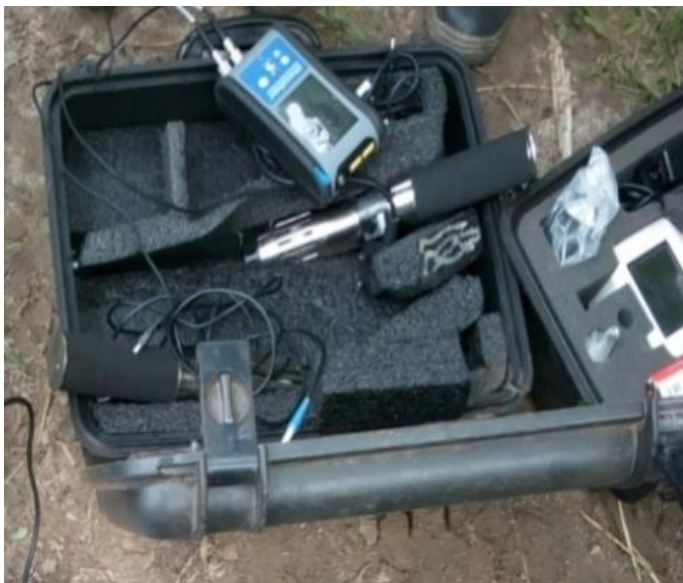
Plate 6.1: Air quality Equipment (Casella Cel Micro Dust Pro 880nm)
