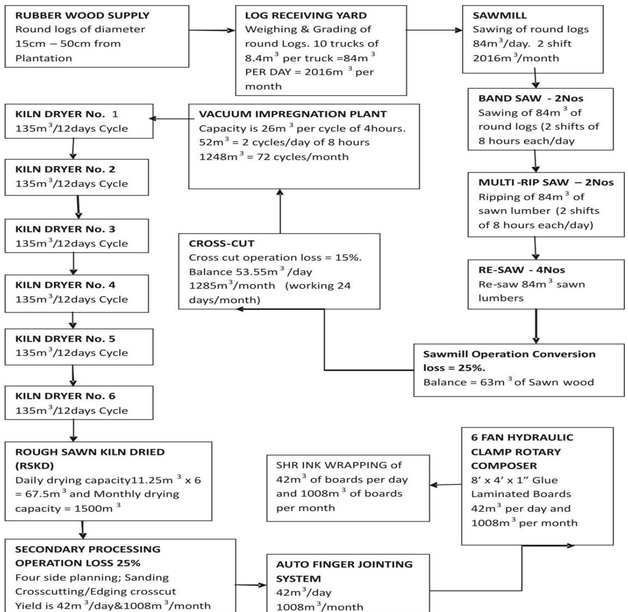
Figure 3.4 Process description of the proposed project
