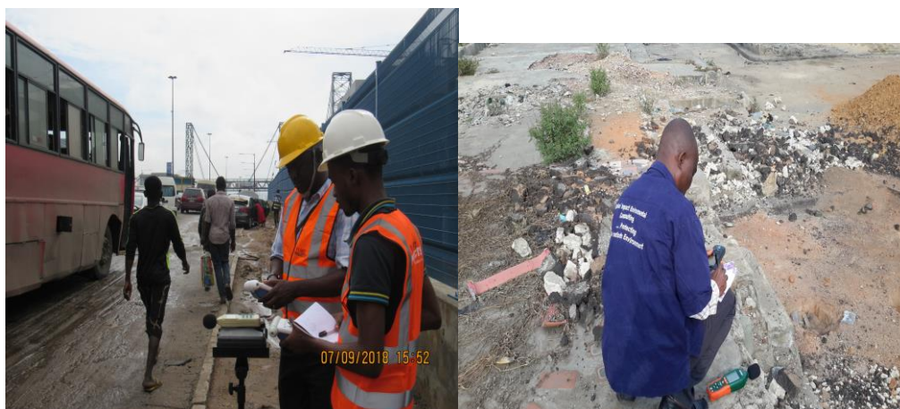
Plate 4.1: Typical Air Quality/Noise Monitoring Setup during the Study
