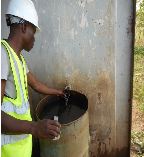
Plate 4.2.8.1a: Water quality sampling from the Angwan- distribution tap of Borehole II, at TCN, Kaduna Sub-Station.
