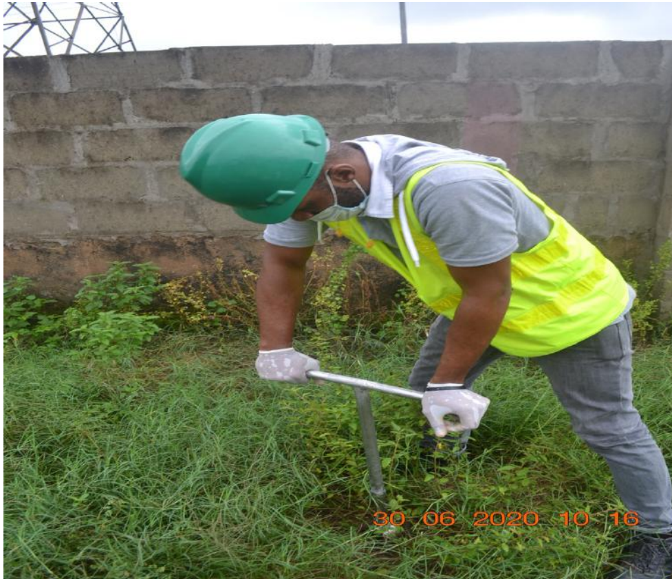
Plate 4.15: Soil sampling using a soil auger by Azmarineberg personnel
