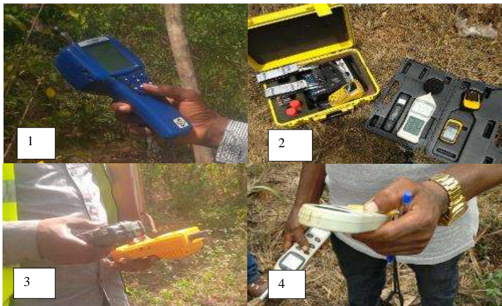
Plate 4.1: Air quality sampling station in the proposed Project location - 1: Particle Counter (SPM), 2: GPS, Test kits, etc., 3: Multi Gas Meter and 4: Noise Meter and Weather Tracker
