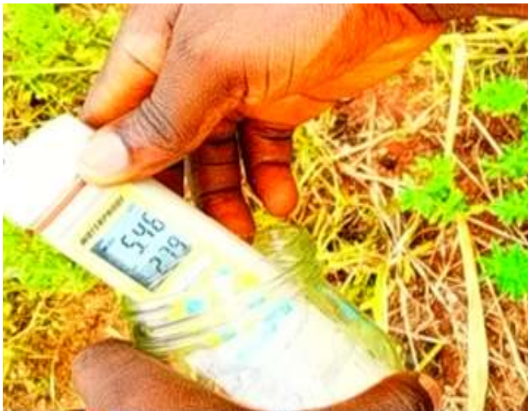
Plate 4.2: pH meter being used for in situ measurement of water quality
