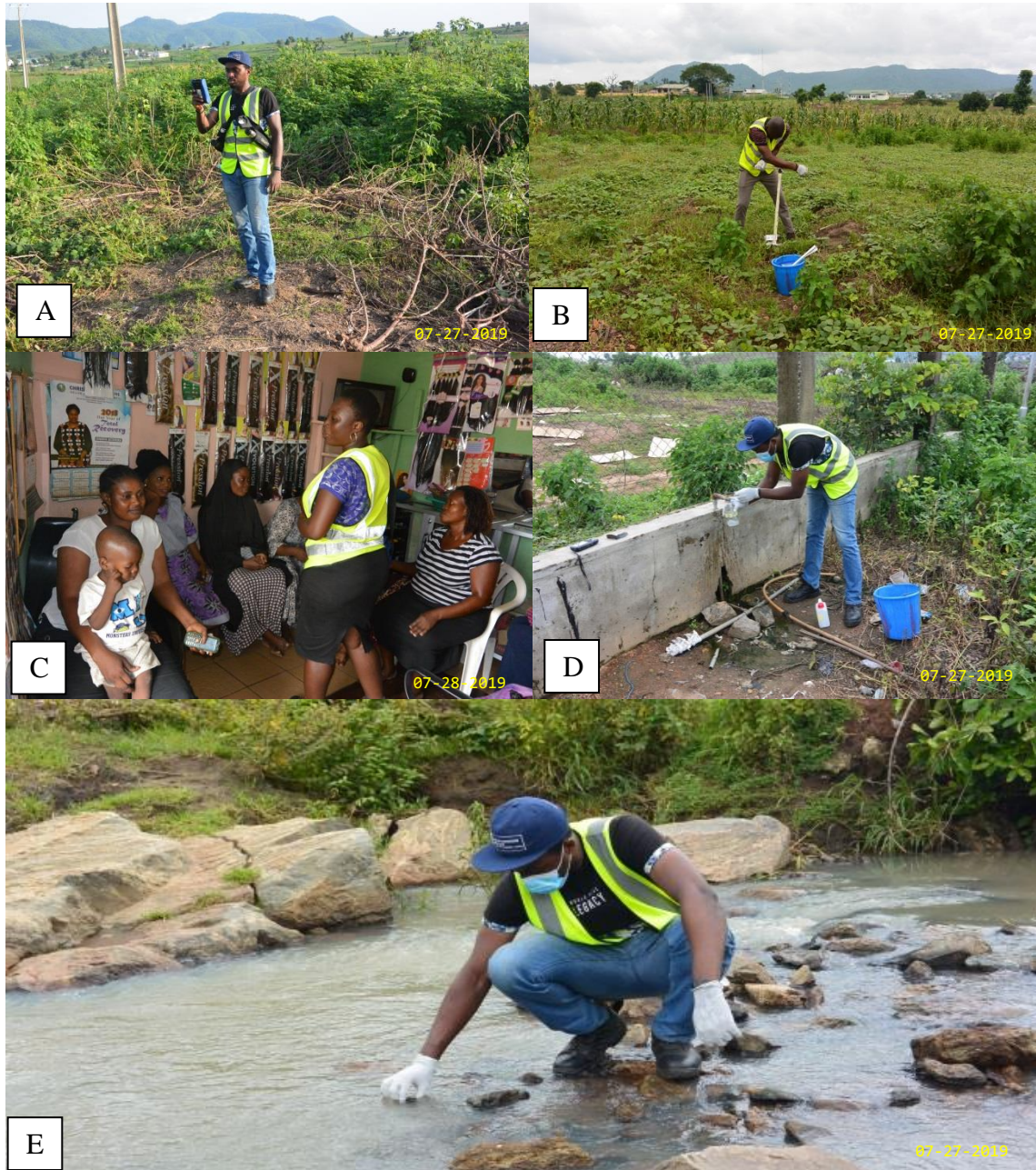
Plate 4.1: Sample Photographs of field sampling activities at the study area: A- Noise/Air sampling, B- Soil sampling, C- Socio-economic survey, D- Groundwater sampling, E- Surface water sampling
