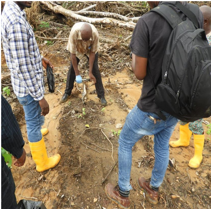
Plate 4.6.1: Collecting Core Soil Samples with a Soil Auger at Study Area
