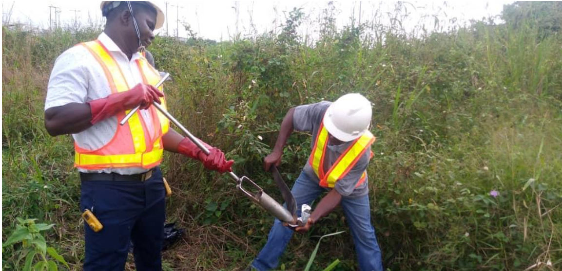
Plate 4.3: Soil sampling showing 3 cores where representative samples were collected
