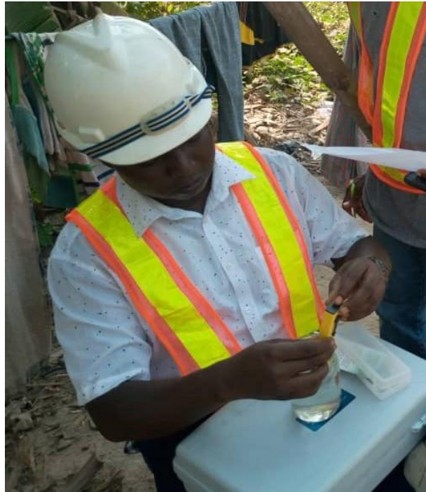
Plate 4.2a: Taking of Groundwater Samples/pH meter being used for in situ measurement of water quality
