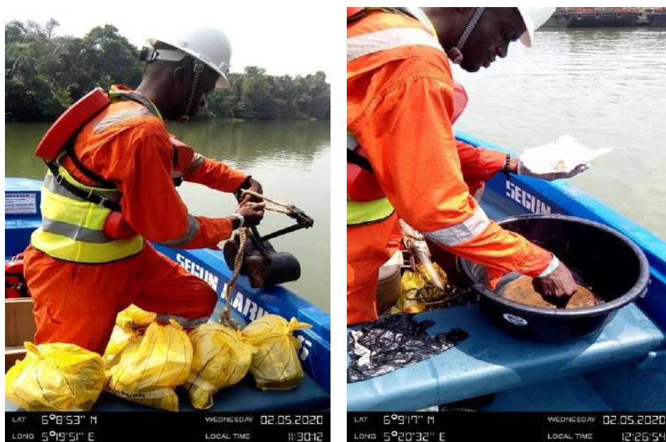
Plate 4.4: Sediment Sampling and Sample Preparation
