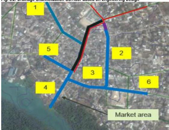
The Road Sections shown in red, black and blue in Figure 6.2 are the primary corridors proposed for the flood control channelization. These road sections are also marked as 1, 2, 3, 4, 5, and 6. Table 6.1 describes these Road Sections and the nature of the works to be carried out along each corridor.
