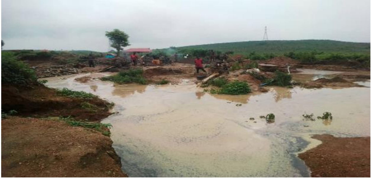
Processing of gold/ wolframite from the gold ore with chemicals and the pollution of water bodies
